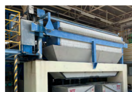
Automated backwashing disc filter equipment at TOTO (Thailand)
